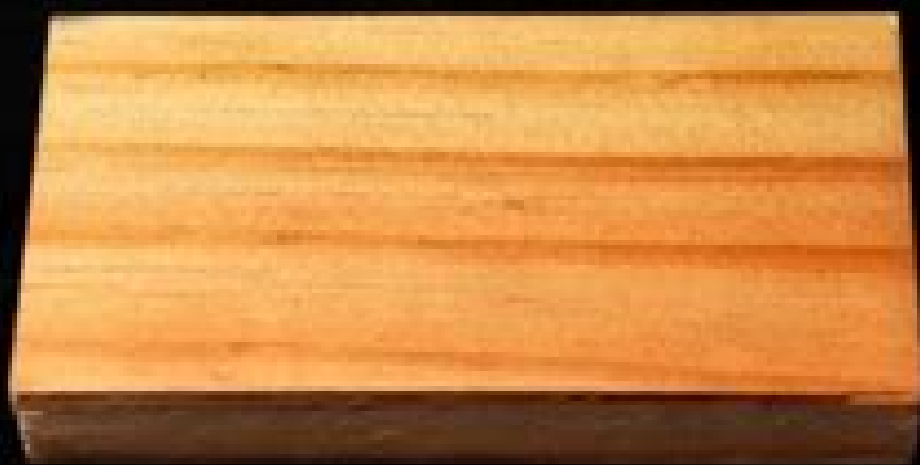
1 Coat of Polyurethane
